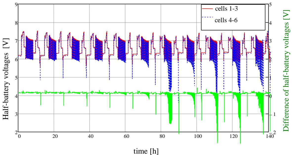
Figure 6: Comparison of the half-battery voltages. The difference between the two half-cell voltages (lower curve) increases drastically at the end of life.
