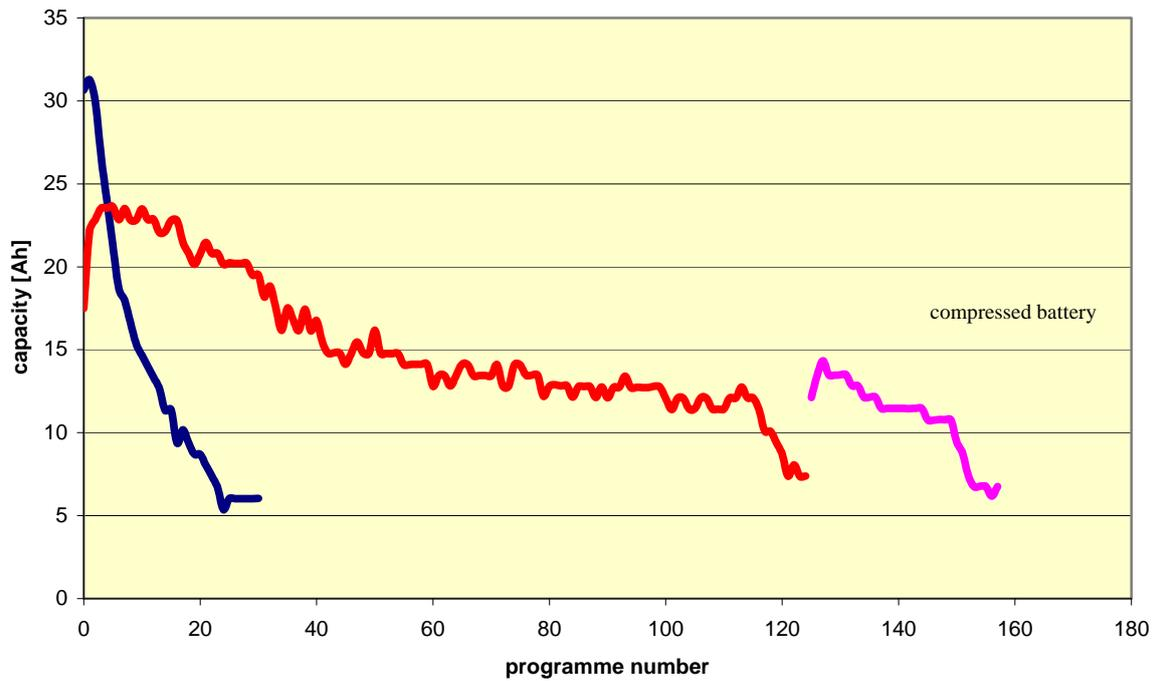
Figure 5: This diagram shows the (poor) result with a conventional battery (with pocket-type separators) and a charge voltage of 15 V, at left, and the (much better) result of the valve regulated battery with glass mat separators. The compressed VRLA-battery achieved more programmes than the uncompressed battery.
