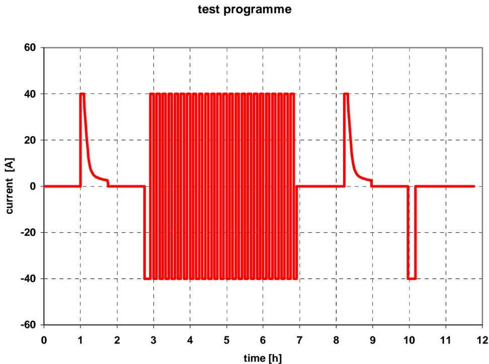
*Figure 4: The test programme starts with a full charge, followed by 25 partial discharges and 24 partial charges, and finally a full charge and a full discharge. The charge and discharge current was 40 A.*
