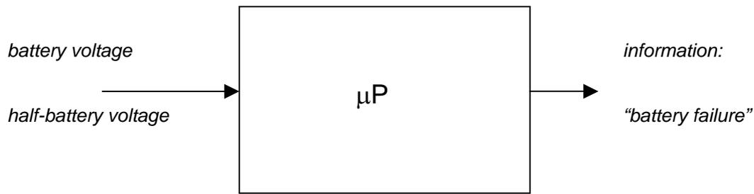
Figure 1: Principle of the battery failure detector. A microprocessor is used for the measurement and it compares the half-battery voltages.
