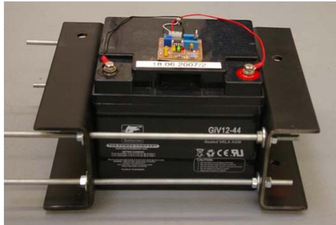
*Figure 3: Device to maintain a sidewall mechanical compression, using disc springs. On the top of the battery one recognises the failure detector.*
